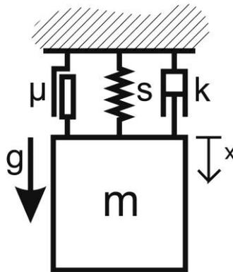
**Figure 15:** Simplified viscoelastic model of fabric behavior
